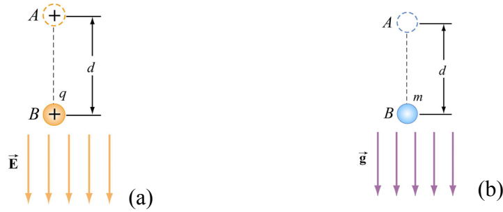
Figure 3.2.1 (a) A charge q which moves in the direction of a constant electric field \vec{E} . (b) A mass m that moves in the direction of a constant gravitational field \vec{g} .
