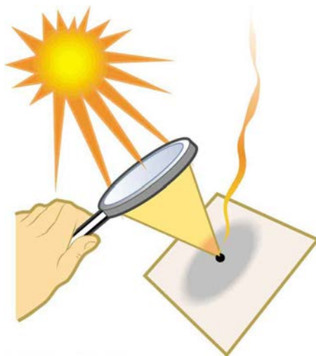
Figure 25.28 Sunlight focused by a converging magnifying glass can burn paper. Light rays from the sun are nearly parallel and cross at the focal point of the lens. The more powerful the lens, the closer to the lens the rays will cross.
