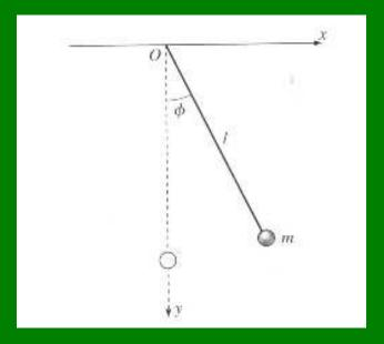
The bob moves in both the x and y directions (but it is constrained by the rod)
