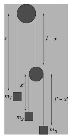
The system now has two degrees of freedom its instantaneous position is specified by the two coordinates  $\boldsymbol{x}$  and  $\boldsymbol{x'}$
