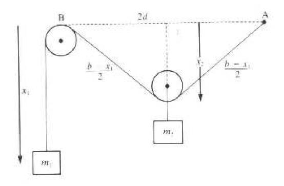
A light string of length b is attached at point A, passes over a pulley at point B located a distance 2d away, and finally attaches to mass  $m_1$ .
