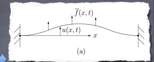
Let u(x,t) denote transverse displacement where x is distance from left end and t is time Force distribution (of dimension force/length<sup>2</sup>) denoted  $rac{f}(x,t)$ We assume that all motion is vertical and displacement u and slope  $\theta = \partial u / \partial x$  are both small For small  $\theta = \sin \theta \approx \tan \theta$
